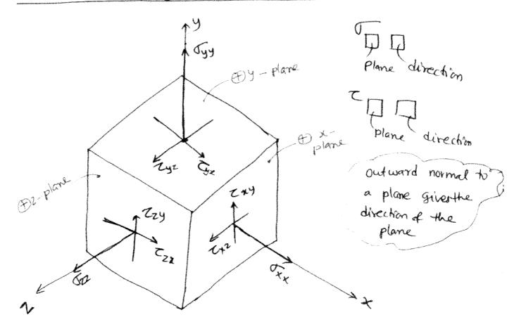
→ At any point under general loading condition no. of stress?
