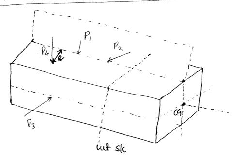
$\rightarrow$  P<sub>1</sub>, P<sub>2</sub>, P<sub>3</sub> & P<sub>4</sub> are external forces applied by some external agent (outside the beam).
